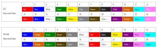
The above chart is a quick reference guide for indentification of fibers and tubes in the most common cable designs. For detailed information about the color code systems, please contact Hexatronic.
